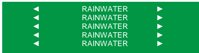
FIGURE 7.1 CONTINUOUS GREEN PIPE MARKER FOR PIPEWORK LESS THAN 40 MM DIAMETER (USED TO IDENTIFY RAINWATER PIPEWORK)
